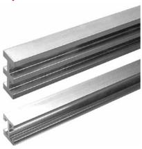
Use in higher-current applications between 756 A and 2,000 A (please contact Hoffman regarding how to achieve 4,000 A). The outer-most section of these symmetrical profile busbars are 30 x 10 mm. All 60-mm system components can be mounted on systems using this busbar structure.
