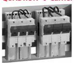
Busbar mounted 3-pole fuse holder for UL Listed Class J 30 and 60 A ferrule size fuses. Holders are offered with or without open fuse indication. In indication units, the LED indicator lamp will glow when the fuse is open. Indicator units operate at voltages between 110 and 600 V. Complete solution on busbar adaptor, 3-pole for all busbars. QUADRON J-Carrier is a trademark of Wöhner GmbH & Co. KG.
