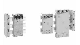
Adapters configured specifically for many of the industry's leading molded-case circuit breakers. The hole pattern for the mounting screws, pitch and length of the terminal connections are specific to the breaker they are designed to mount.
