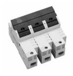
DIN Rail mountable fuse holders for 30 and 60 A ferrule size UL Class J fuses. Offered in single pole, 2-pole or 3-pole configurations with LED open fuse indication. Indicator operates on systems between 110 and 600 V. The LED lamp will glow when the fuse is open (blown). Holders meet IP20 touchsafe design standards.
